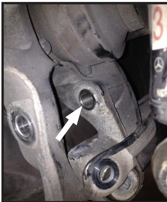
13. REINSTALL AND TIGHTEN THE LOWER CONTROL ARM BOLT. (FIGURES 66, 67)
